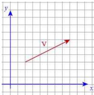
The rectangular coordinate notation for this vector is  $\mathbf{v} = \langle 6, 3 \rangle$  or  $\vec{v} = \langle 6, 3 \rangle$ . Note the use of **angle brackets** here.
