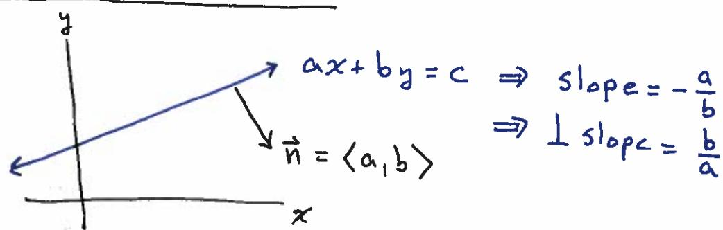
So the line with equation  $ax + by = c$  has a normal vector  $\vec{n} = \langle a, b \rangle$ .
