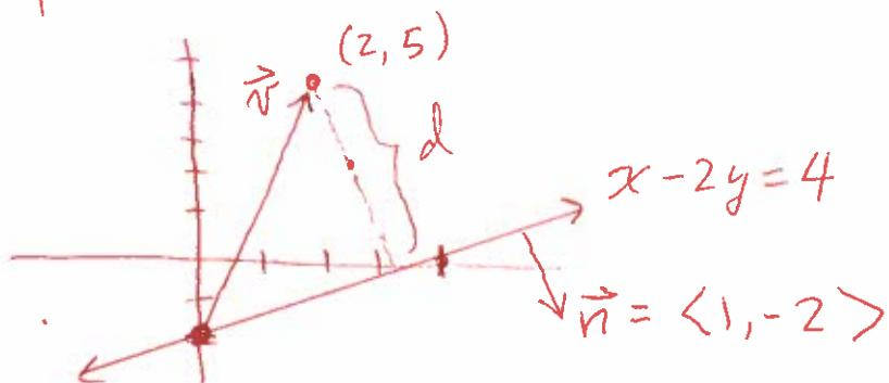
We get  $\vec{n}$  from the  $x$  and  $y$  coefficients of the equation of the line in standard form. Next pick a point on the line, say  $(0, -2)$  and form the vector  $\vec{v} = \langle 2, 7 \rangle$  as shown. Then the orthogonal distance is
