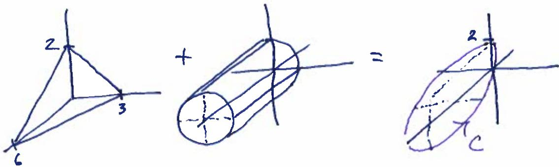
The curve  $C$  bounds the part of the plane  $x=6-2y-3z$  that is inside  $y^2+z^2=4$
