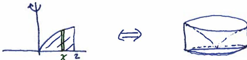
$$\left. \begin{aligned} dA &= \sqrt{x} dx \\ R &= x \end{aligned} \right\} \Rightarrow dV = 2\pi x \sqrt{x} dx$$
